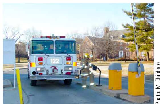
Figure 3.14. An entrance to a private fire lane. The delays caused by electronic gates can be minimized by providing the fire service with access cards or remote access controls.
